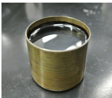
Container with asphalt
